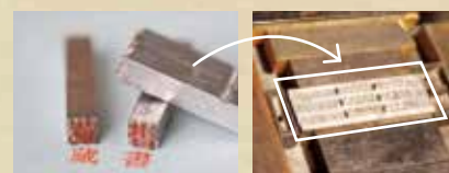
Metal type. The kanji characters are mirrored. The characters are arranged in lines.
